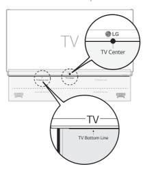
3 With a pen, mark screw holes on the installation guide where the wall brackets will be attached.
