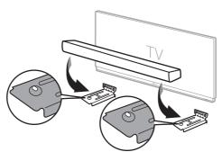
8 Firmly attach the product to the wall brackets using the screws provided.
