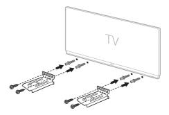
7 Place the product on the brackets. Position the product on the brackets so the screw holes on the bottom of the product align with the screw holes on the wall bracket.
